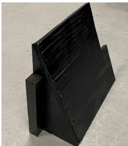
Cable protective panel assembled
