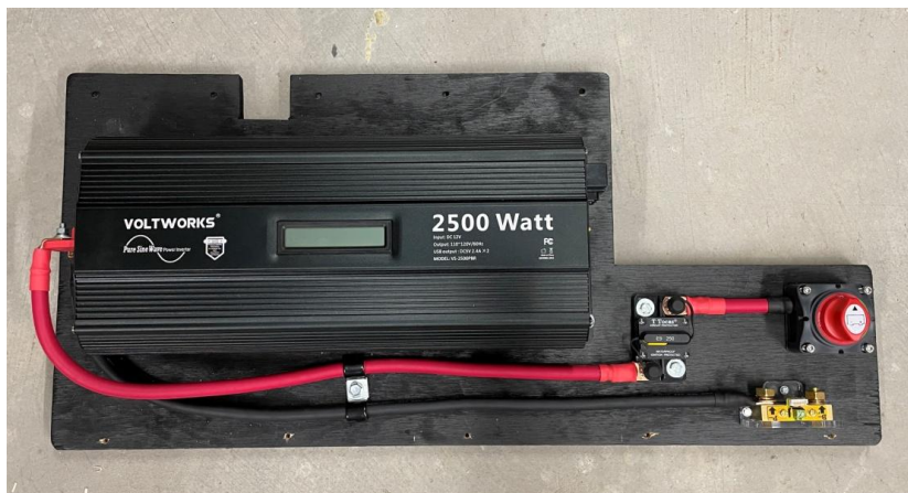
Inverter module complete and ready to mount
