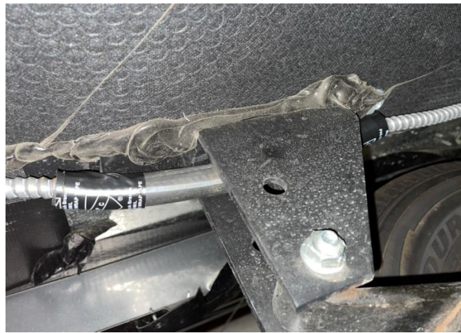
Using 1/2" ID heater hose to sheath MC cable around metal
