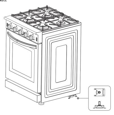
4 Open the storage drawer, slide the notches on the front brackets over the front feet, then screw the brackets into the floor using two of the provided screws for each bracket.
