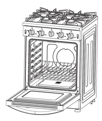
2 Remove the racks from the oven. To remove a rack, pull the rack toward you until it reaches the stop position, then tilt the front edge of the rack up and pull the rack completely out.
