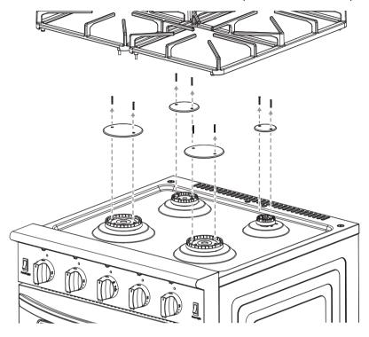
3 Remove the two screws on the burner base cap, then remove the cap and burner base.
