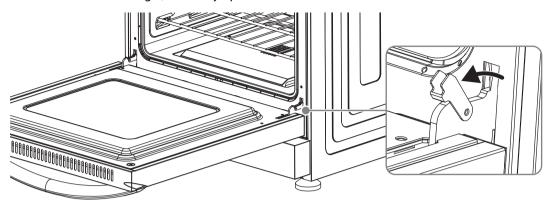
**2** Gently close the door about halfway to disengage the hinges, then pull out the door and place it on a protected surface.
