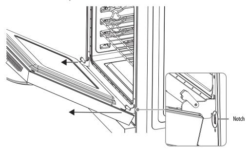
2 Carefully close the door. If the door does not easily close, do not force it. Make sure that the hinges are correctly installed.
