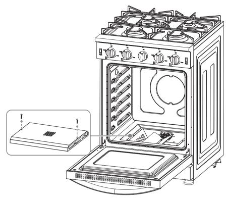
4 Remove the two screws from the pilot lamp and the single screw on the tube burner, then lift the lamp and burner up and out of the oven.
