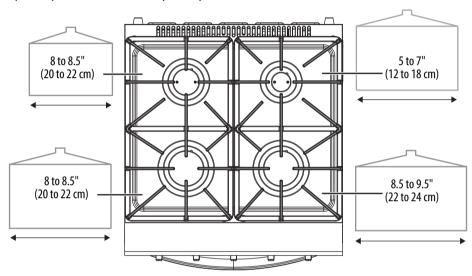
Normal burner (mid-size): 8 to 8.5" (20 to 22 cm) back left Auxiliary burner (small): 5 - 7" (12-18 cm) back right Normal burner (mid-size): 8 to 8.5" (20 to 22 cm) front left Rapid burner (large): 8.5 - 9.5" (22-24 cm) front right
