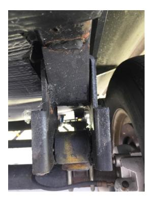
Note that one leg of the V Clip is welded to the forward inner hanger side and the other leg is welded to the aft outer side
