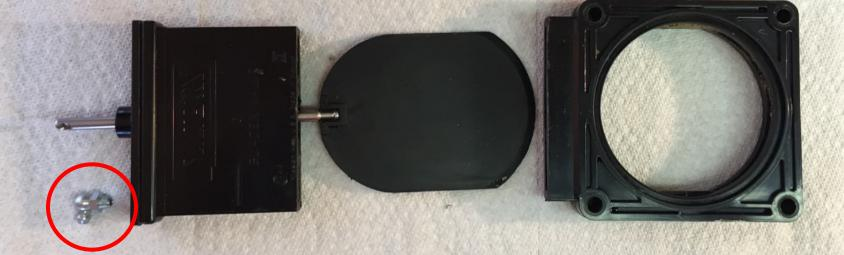
The waste tank gate valves pulls back into a sealed cavity
