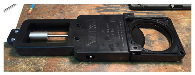
A 3/4" clearance opening is drilled in the removable outer shell and a 1/8" PT hole is drilled and tapped into the body of the gate valve for the zerk grease fitting.
