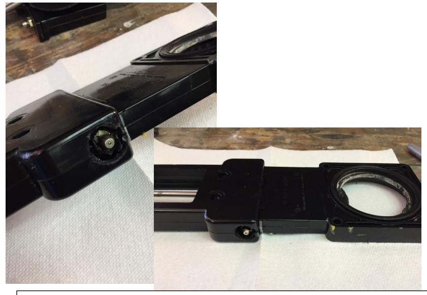
After the first prototype, I discovered that I had to move the grease fitting "around the corner" to clear the cable attaching bracket
